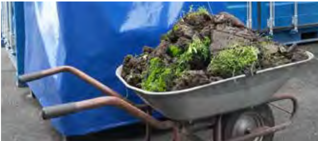
Residual sludge volume after dewatering of 5 m 3 activated sludge over a period of 3 months. KLARO One system, KLARO SBR tank system
